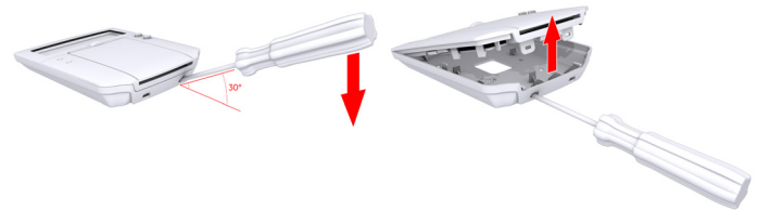
Figure 1: Opening the K641+
